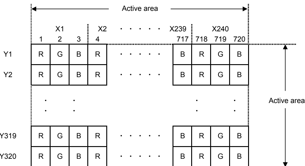
Dot arrangement (FPC cable placed left side)
