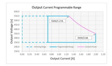
**Note:** EUCO ARENA SPORT 2K1 series can be programmed with wide output current through computer and programming tool. For more details, please refer to DALI programming User Manual or RDM/DMX programming User Manual.
