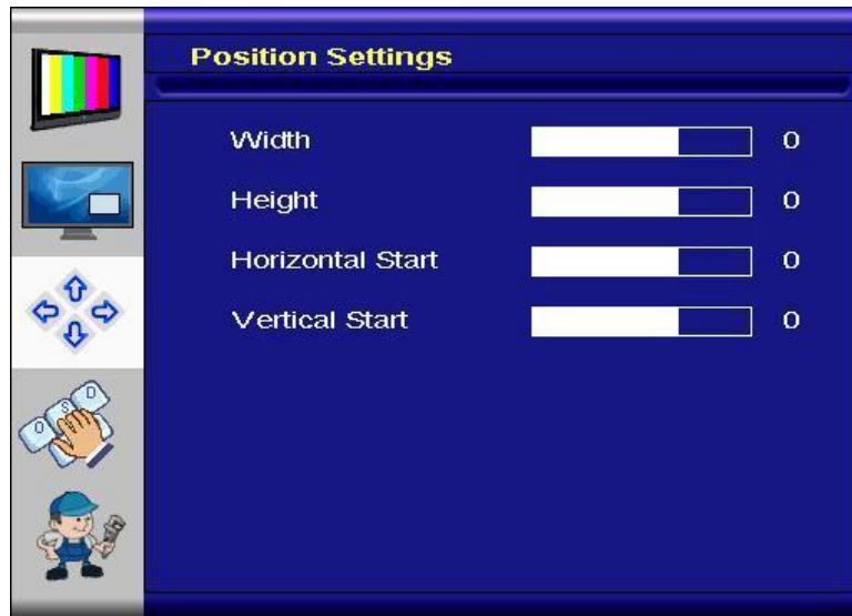
Figure 7.3.a: “Position Settings” menu for video mode of HDMI, S-Video, composite and component inputs.
