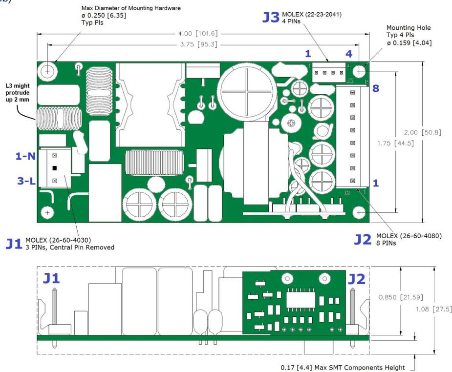
**Forced air cooling: Air flow direction, longitudinal or transverse, must be coplanar to the PCB no matter its orientation.**
