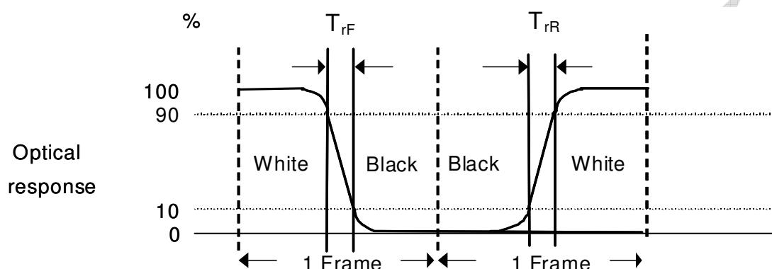
$$T_{rR} + T_{rF} = 12 \text{ msec (typ.)}$$
